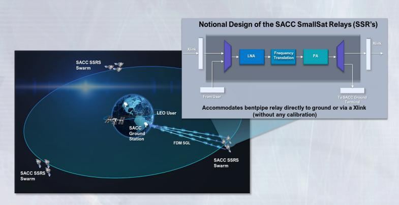
O All the complex Beamforming Functionality is off-loaded to ground processing
