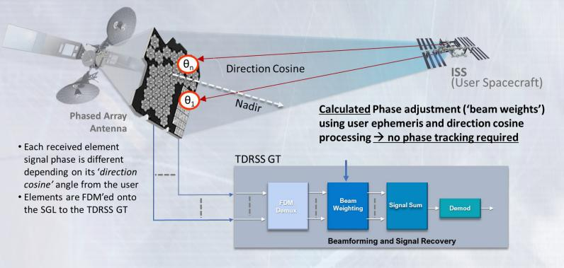
Before we further discuss our unique SACC beamforming, it is important to gain additional insight into traditional phased array beamforming wherein the array elements are attached onto an array frame structure with known and unchanging array 'geometry' like in a TDRS.
